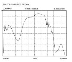
The Model 50 Picoprobe® bias T provides a direct low resistance DC path for supplying up to 1.5 A to a device under test. The bias T also has special circuits which add loss at frequencies below the cut off frequency (26.34 GHz) of WR-22 waveguide. This data was taken by launching a, 40 MHz to 50 GHz, signal from the tips of a calibrated Model 67A into the tips of a Model 50-GSG-150-BT. Without this low frequency loss, most active devices will oscillate.
