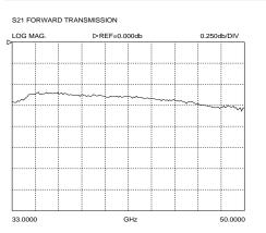
Typical insertion loss of a Model 50-GSG-100-BT
