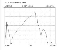
The Model 75 Picoprobe® bias T provides a direct low resistance DC path for supplying up to 1.5 A to a device under test. The bias T also has special circuits which add loss at frequencies below the cut off frequency (39.86 GHz) of WR-15 waveguide. This data was taken by launching a, 40 MHz to 67 GHz, signal from the tips of a calibrated Model 67A Picoprobe® into the tips of a Model 75-GSG-150-BT. Without this low frequency loss most active devices will oscillate.
