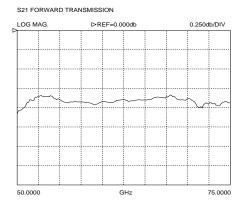
Typical insertion loss of a Model 75-GSG-100-BT
