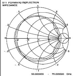
Forward reflection into an open ended 50 ps coplanar line after a one port SOLT calibration was performed using our CS-5 calibration substrate. The smooth inwardly spiraling line shows the increasing loss of the 50 ps coplanar line with frequency, coupled with a smoothly changing phase.
