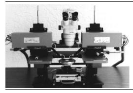
Micropositioners are available to hold Wiltron V band modules so that the module and the probe are micropositioned as a single unit. In this way, total ease of positioning can be achieved with minimum insertion loss.
