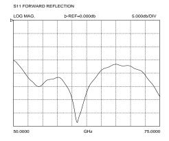
Typical uncalibrated performance of a Model 75-GSG-100-BT while touching a 50 ohm load on our CS-5 calibration substrate.
