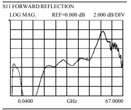
The Model 120 Picoprobe bias T provides a direct low resistance DC path for supplying up to 1.5 A to a device under test. The bias T also has special circuits which add loss at frequencies below the cut off frequency (59.05 GHz) of WR-10 waveguide. This data was taken by launching a, 40 MHz to 67 GHz, signal from the tips of a calibrated Model 67A into the tips of a Model 120-GSG-150-BT. Without this low frequency loss most active devices will oscillate.
