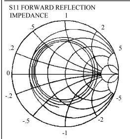
Forward reflection of a Model 120 into an open ended 50 ps coplanar line after an LRM calibration was performed using our CS-5 calibration substrate. The smooth inwardly spiraling line shows the increasing loss of the 50 ps coplanar line with frequency, coupled with a smoothly changing phase.
