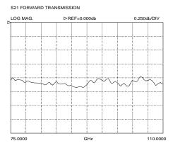
Typical insertion loss of a Model 120-GSG-150-BT
