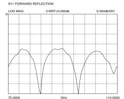
Typical uncalibrated performance of a Model 120-GSG-150-BT while touching a 50 ohm load on our CS-5 calibration substrate.
